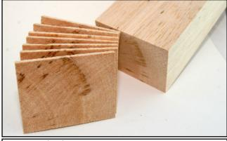
SPECIAL (EG) END GRAIN BALSA CORE CONSTRUC-TION MAKES FOR A STIFFER BLADE WITH NO SUR-FACE COMPRESSION. RESULTING IN SPEED!!!
