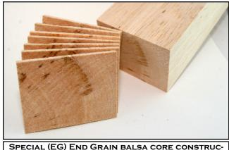
TION MAKES FOR A STIFFER BLADE WITH NO SUR-FACE COMPRESSION. RESULTING IN SPEED!!!
